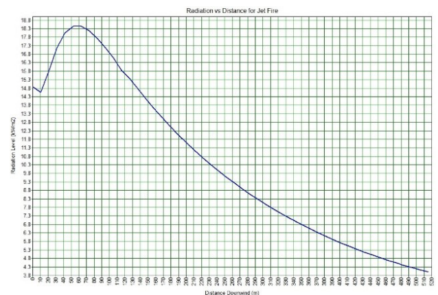
Figure 17. Max of intensity is 18.5 (kw/m 2 ) for open valve mode
