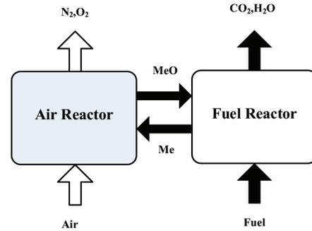
Figure 1. A schematic view of chemical looping combustion
