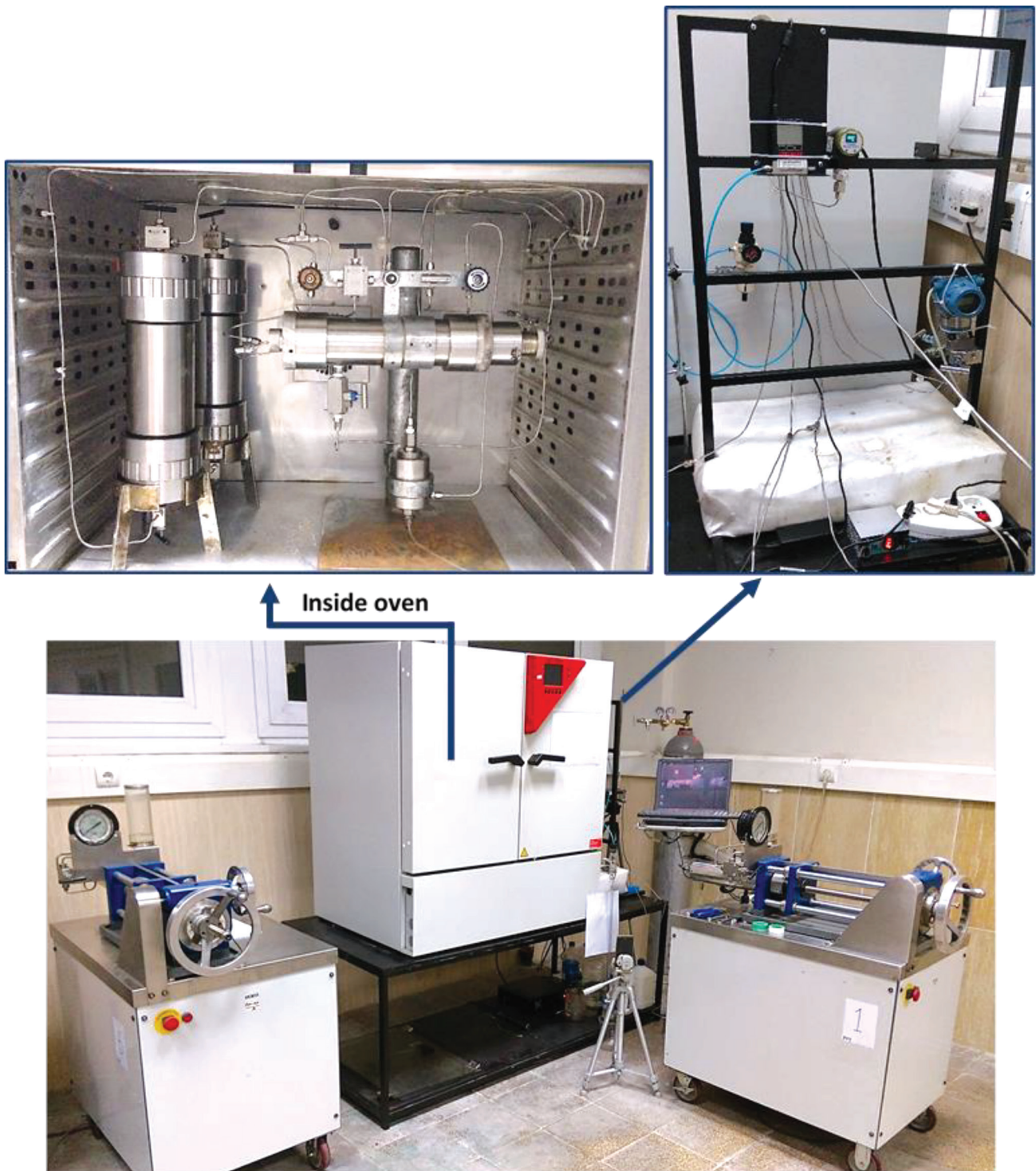
Fig. 1. Experimental set up for core displacement tests and chemical treatment.
