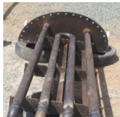
Figure 2. A real photograph of heating coil
